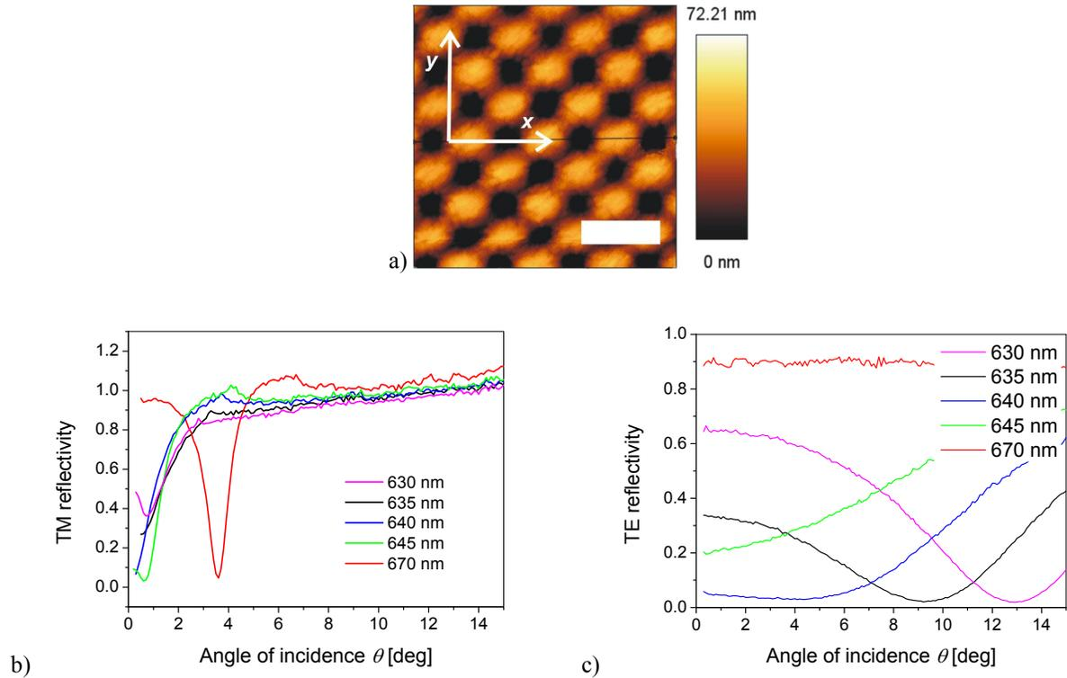
Figure 3. AFM characterization of grating morphology (a scale bar length of  $0.6 \mu\text{m}$ ) and b) TM and c) TE angular reflectivity spectrum for the prepared plasmonic chip with the SU8 layer coating (thickness  $t_{\text{SU8}}=12$  nm).
