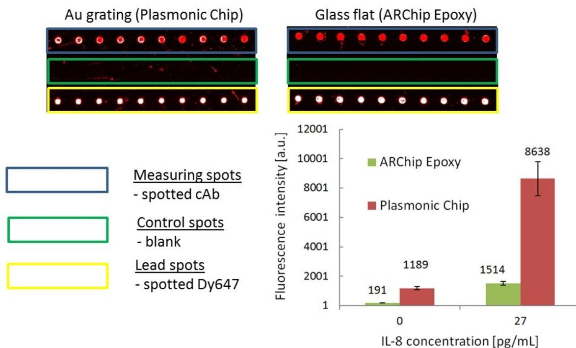
Figure 4. Example of fluorescence images for IL8 assay on microarrays spotted on developed Au grating (plasmonic chip) and regular (ARChip Epoxy) slides with measuring, control and lead arrays of spots (upper part). Comparison of fluorescence signal for the IL-8 assay is showed at the bottom.
