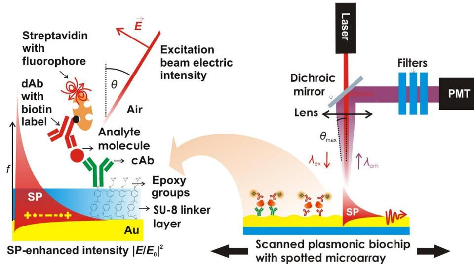
Figure 2. Schematics of prepared sensor chip for epi-fluorescence detection with an interface architecture for sandwich assay detection format.
