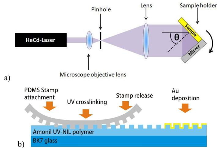
Figure 1. Schematics of a) laser interference lithography setup for the preparation of crossed relief grating master and b) the preparation of replicas for the plasmonic amplification of fluorescence signal by using soft lithography.
